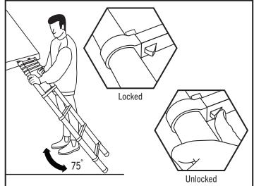
2. Adjust to the correct height by unlocking the top rungs and sliding up. Ensure each rung is locked before using (see locking positions above). Position the ladder at a 75° angle to the ground.
