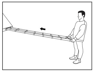
1. When collapsing the ladder, hold the bottom rung and press the left and right release buttons. Hold the ladder frame - not the rung when pressing the release buttons.
