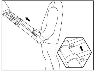
2. Slowly and sequentially collapse the ladder from the lowest rung to the top.
