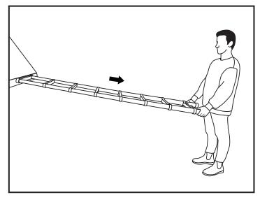
1. When opening the ladder, slowly and sequentially extend the ladder from the top to the bottom, until fully extended.
