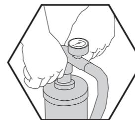
5. It is recommended in hot weather that 6psi is used to allow for the air to expand inside the air tubes. In cooler/windier conditions 8psi is recommended. Please adjust the pressure in the air tubes as the ambient temperature changes. Only use the pump provided as it has a pressure gauge which shows the recommended pressure (psi).
