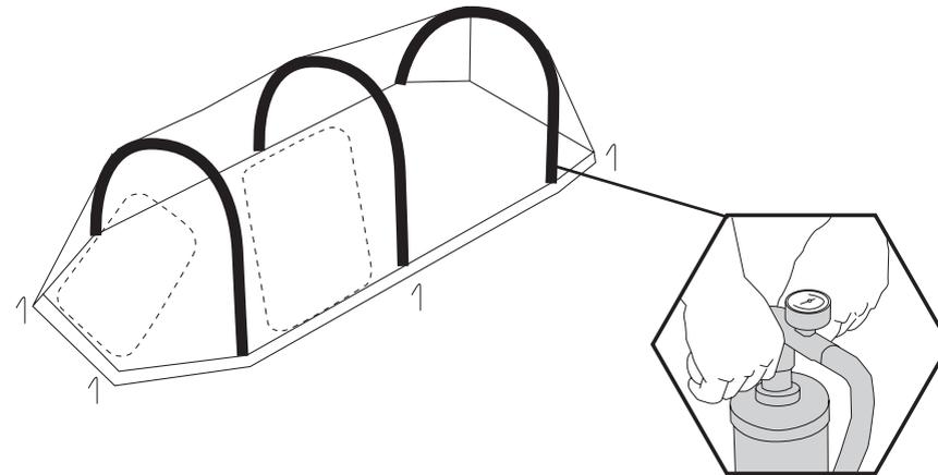
6. It is recommended in hot weather that 6psi is used to allow for the air to expand inside the air tubes. In cooler/windier conditions 8psi is recommended. Please adjust the pressure in the air tubes as the ambient temperature changes. Only use the pump provided as it has a pressure gauge which shows the recommended pressure (psi).
