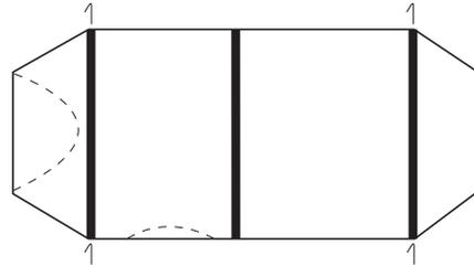
2. Pitch so the tent is in line with wind, never side on. Spread out the tent and peg out the four main corners ensuring the tent is pulled taut and square. Then peg out the remaining pegging points.
