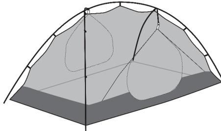
5. Carefully pull the fly over the top of the inner and peg out the four corners. Opening both doors, reach under the fly and attach any Velcro ties to the poles. Once this is done, zip up the doors and finish pegging out the fly.
