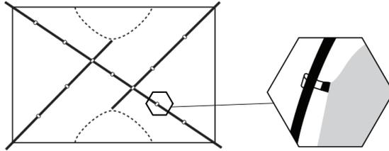
4. Take one of the remaining RED poles and fit a pin and ring with RED webbing into the pole. Clip the other end of the pole into the eyelet with the RED webbing above the opposite door. Clip on the speed clips. Repeat with the second RED pole.
